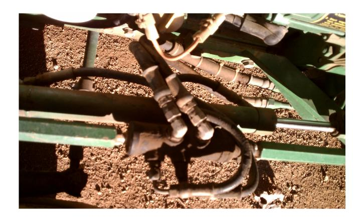
4 Hydraulic hoses need to be replaced. Basically dry rotted.
